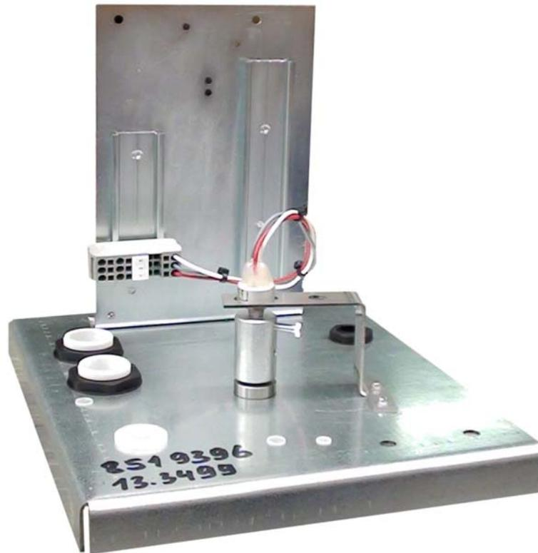
The *steering tower box* continuously monitors the steering movements and simultaneously limits the maximum steering angle. The sensor is connected to the rotatable pusher part via an adapter sleeve. Make certain that the screw on the adapter sleeve is firmly tightened; otherwise the machine will not register any steering movements.
